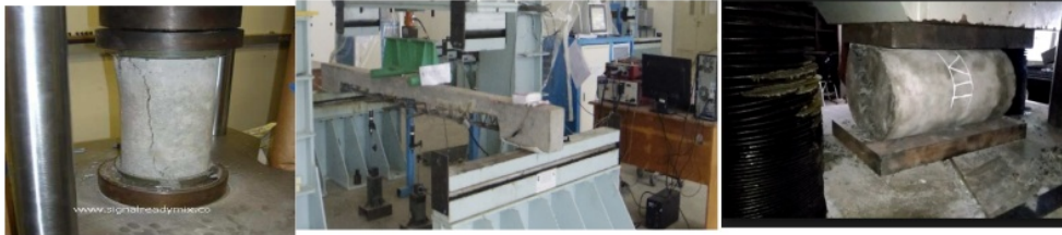
Uji Tekan (ASTM C39)
